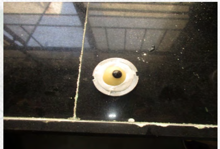
Fig 5: Invested wax pattern
